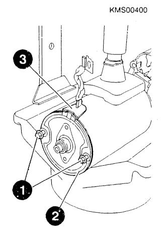
Assembling commutator end shield
